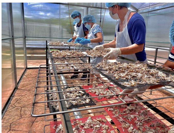
Figure 4. Filling solar dryer with fish waste.
