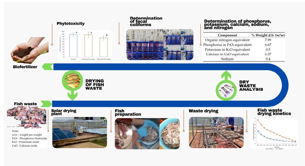
Figure 1. Production of biofertilizer based on fish waste through solar drying.
